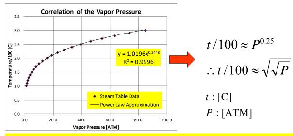
This indicates that an approximate value of the saturated temperature can be obtained by taking the square root of the square root of the saturated vapor pressure in [ATM], and then multiplying the result by 100.
