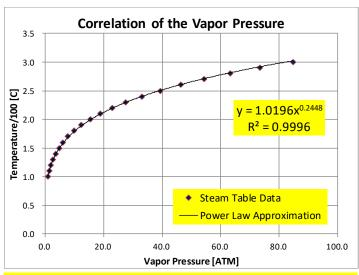
A highly accurate correlation can be obtained by plotting the temperature/100 [C] versus the vapor pressure [ATM] and using the power law approximation.
