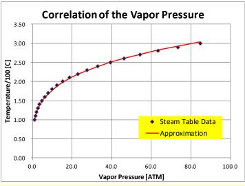
Below 300C [85 ATM], it can be seen that the deviation is around  $\pm$  1%. Even in near the critical point, the deviation is 3% or less, which is not that much different than the Antoine equation.
